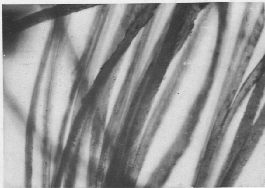
Fig. 4 - Microphoto of the silk fibre (warp thread) showing some presence of residual gum sericin (Photo by Mme H. Meyer).
