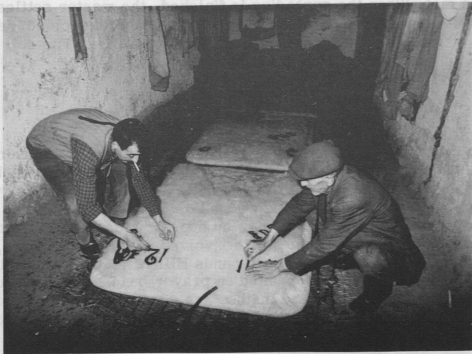
Fig. 4 - Numbering of a kepenek with coloured felt strips after the first stepping of the roll Afyon, workshop of Cemalettin Özçalışan, 1973
