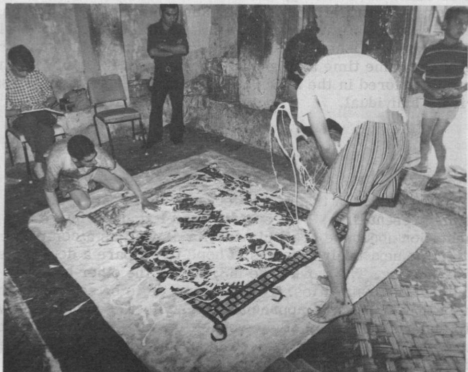
Fig. 8 - Hot water, thick with soap, is spread over a rug during the fulling process Shiraz, workshop of Abdol Ali Oujji, 1973
