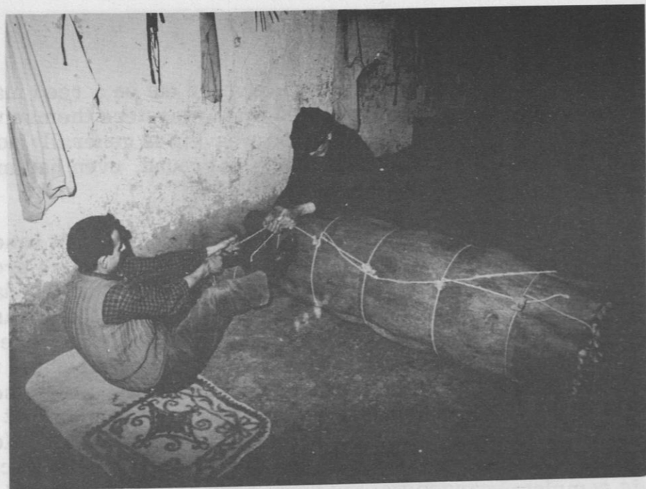
Fig. 3 - The roll is wrapped with a piece of felt and tied tightly Afyon, workshop of Cemalettin Özçalışan, 1973
