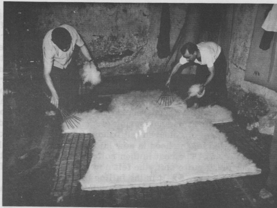
Fig. 5 - The wool of the hood is laid out for a sleeved kepenek after the first stepping of the roll Tire, workshop of Mustafa Elal, 1973
